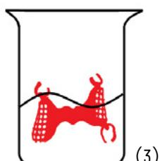
Note: The effectiveness of the cleaning bath diminishes with each use. Therefore, replace the bath if the cleaning effectiveness is reduced. Thoroughly clean the cavities and hollows, if necessary, using compressed air.
